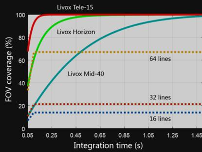
Fig.3 The FOV coverage of Livox LiDAR sensors, including Horizon, Tele-15, and Mid-40; compared with other (non-Livox) LiDAR sensors that used common mechanical scanning methods, with line-number and vertical FOV being 64 lines/27°, 32 lines/41°, 16 lines/30°. During calculation, the FOV is gridded with 5mrad\*5mrad.
